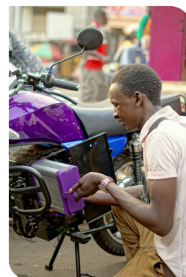
Figure 27: MOPO's battery swap technology. Source: MOPO
