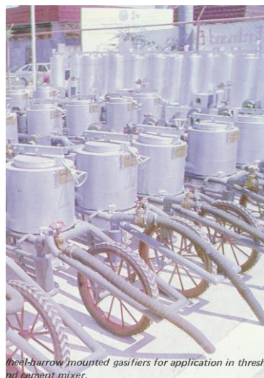
Figure 24. Mass production of GEMCOR gasifiers in the Philippines
