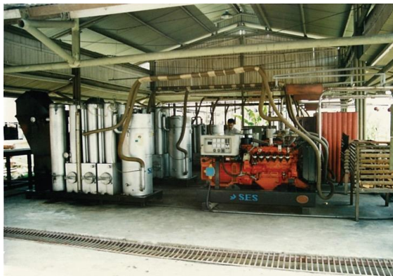
Figure 23. Three Italian made 'SES' gasifiers at a sawmill, Indonesia
