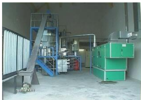
Figure 20. Open-top Xylowatt gasifier at Bulle, Switzerland, based on IISc technology
