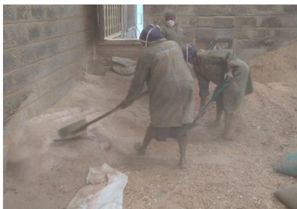
Blending sawdust and condemned maize for briquetting, Kings Biofuels, Murang'a
