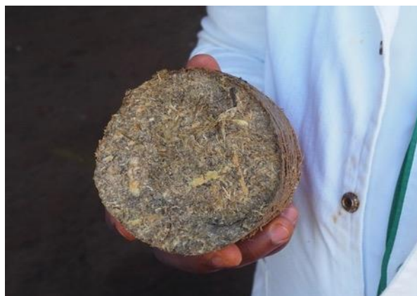
Bagasse briquette from White Coal, Kisumu (photo taken at Makomboki)
