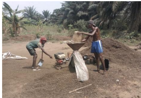
Mechanical cracking of oil palm nuts, Ondo State
